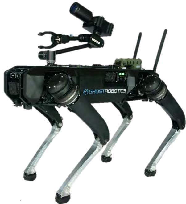
V60 v5 shown with Optional Body Bumpers, Antennas, HDT Arm, Honeywell MultiRAE Gas & Raman Spectroscopy Sensors
