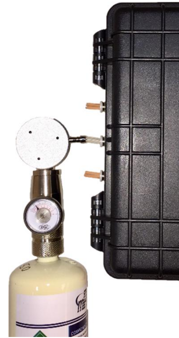
Calibration Gas Connections
